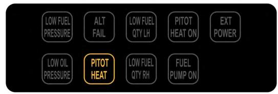
When the Pitot Heating system is activated, the green **PITOT HEAT ON** advisory light turns on and the amber **PITOT HEAT** caution light turns **OFF**, indicating that the Pitot Heating system is functioning properly.
