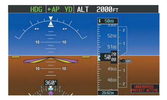
When airspeed increases (as a result of adding power/thrust) to an IAS above 70 KIAS, USP will then disengage and the autopilot will command the aircraft to pitch up until recapturing the vertical reference (vertical vertical flight director mode will switch from white armed to green active).
